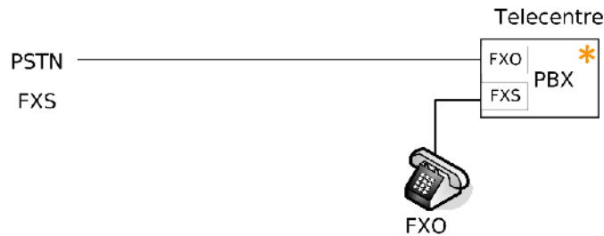
Image 9. The Telecentre uses a TDM400P wildcard to: (1) connect the PBX to the PSTN (FXO module) and (2) route calls to an analogue phone (FXS module).
