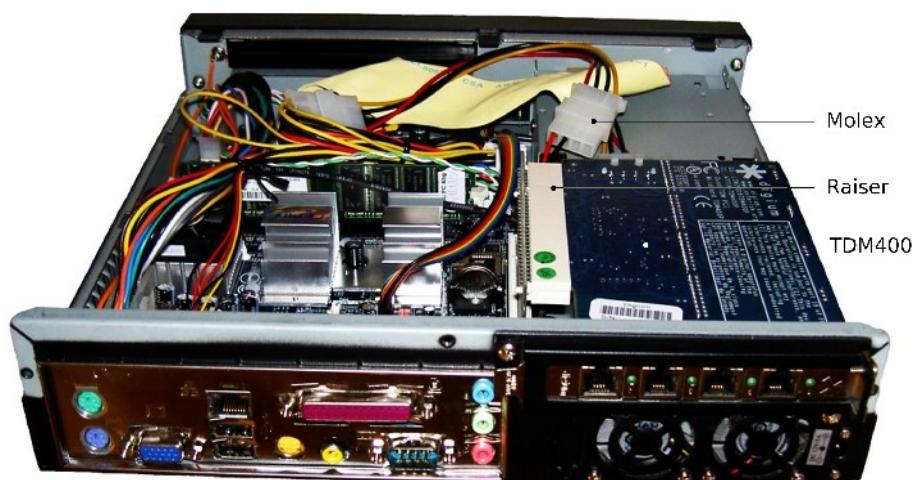
Image 4: A portable PBX running in a mini-ITX board with a Digium TDM400P Card.
