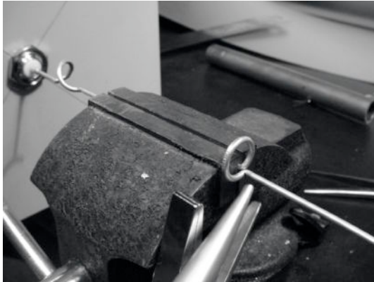
Figure 4.29: Repeat the stretching procedure for all of the remaining coils.
