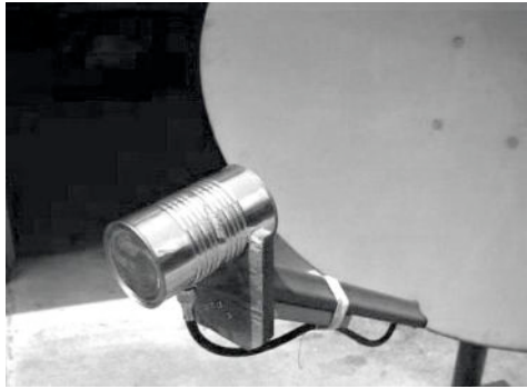
Figure 4.10: Feed horn made from a food can.
