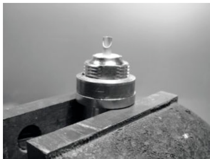
Figure 4.24: Adding a copper pipe spacer helps to match the impedance of the antenna to 50 Ohms.
