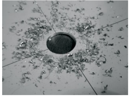
Figure 4.22: Drilling the hole in the metal plate.
