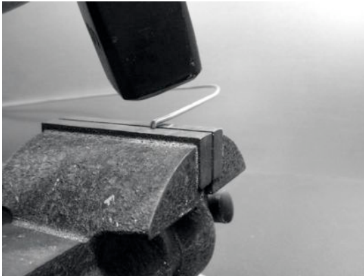
Figure 4.16: Gently tap the wire to make a sharp bend.
