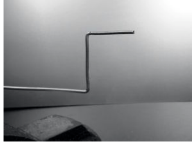
Figure 4.17: Bend the wire into a "Z" shape.
